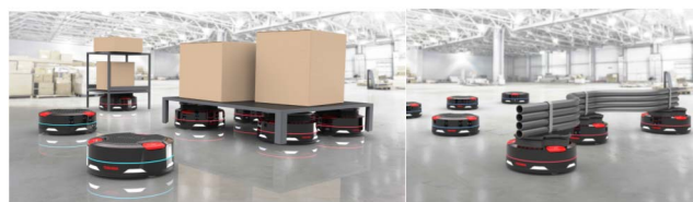
Fig. 1. Vision illustration of the Swarm Testbed for handling pallets with various size and shape.
