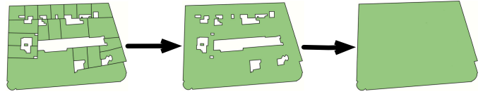
Figure 1. Example of the polygon union operation for a given city block.
