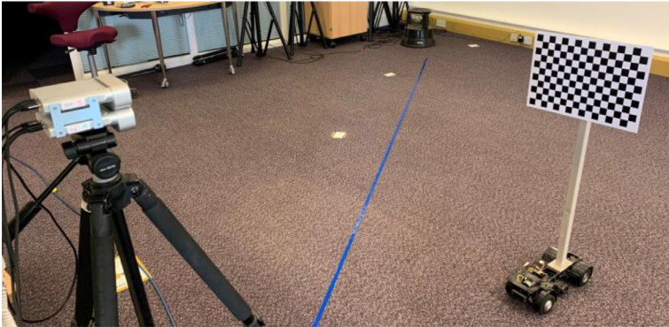
Fig. 5. The calibration set-up used in data collection: the A3 board was attached to a movable stand such that its pose could be easily changed.
