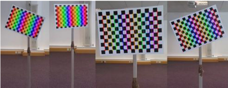
Fig. 6. Sample captures taken during calibration, from the perspective of the Master, after drawChessboardCorners() was applied.
