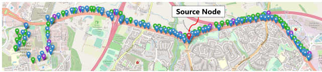
Figure 4: The UMBRELLA network. All nodes are installed on public lampposts across a road of ~7.2km. The red node is our experiment source node. The rest of the nodes are all equipped with an Nordic nRF52840.
