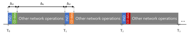
Figure 1: A time-sliced SF control to maximise network resource utilisation. The different data periods represent the different core data patterns.
